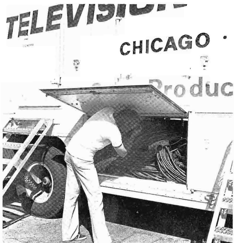
Hundreds of feet of cabling must be carried aboard the van to support a variety of production requirements.
