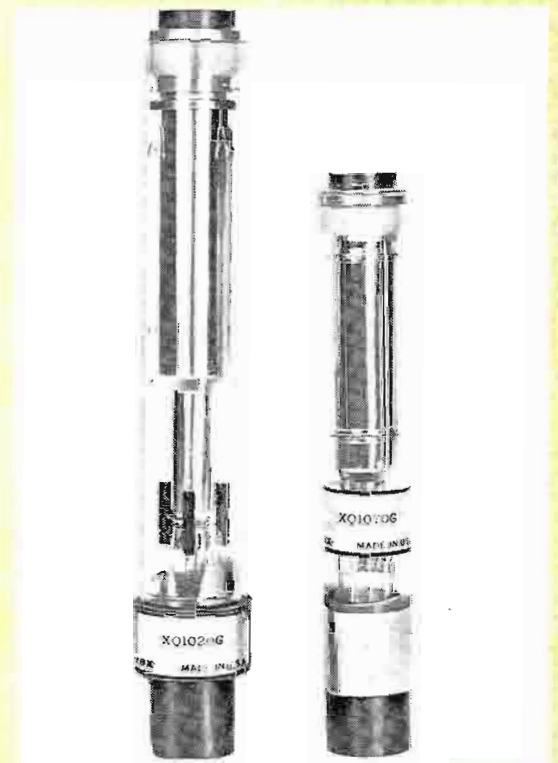
Size comparison between a 30 mm PbO and the one-inch lead oxide type tube used in TKP-45. Advanced video amplifiers in the TKP-45 camera bring signal-to-noise performance of the smaller tube to be equal with the larger tube design.
