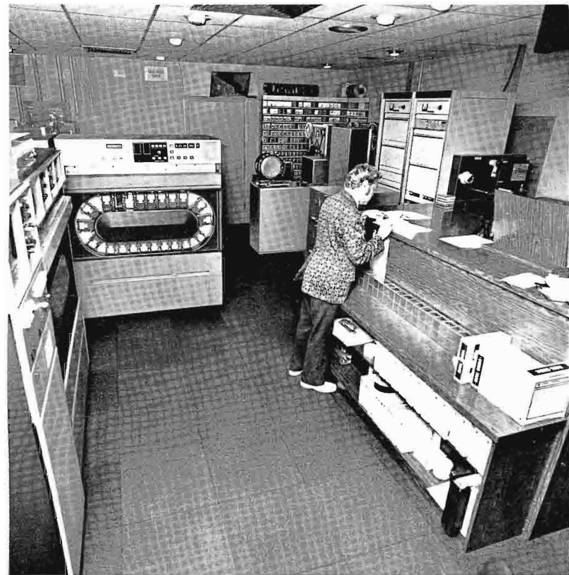
TV-44's two "cart" machines are averaging over 300 plays per day, and are also used for production.
