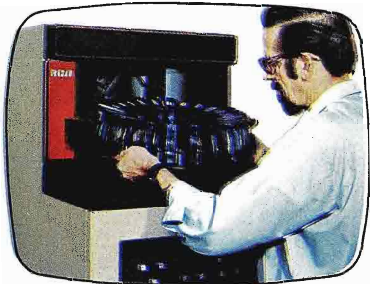
Each cartridge can contain from ten seconds to two minutes of film, with complete cartridge flexibility.
