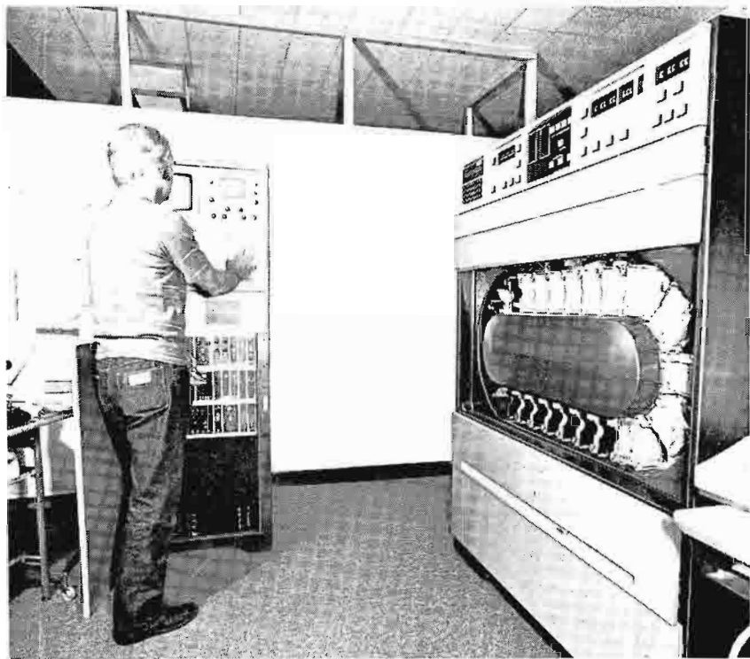
Production TCR-100, equipped with editing accessory, is used for program assembly, for dubbing tape segments of news programs and even as a "master" for making multiple tape dubs.
