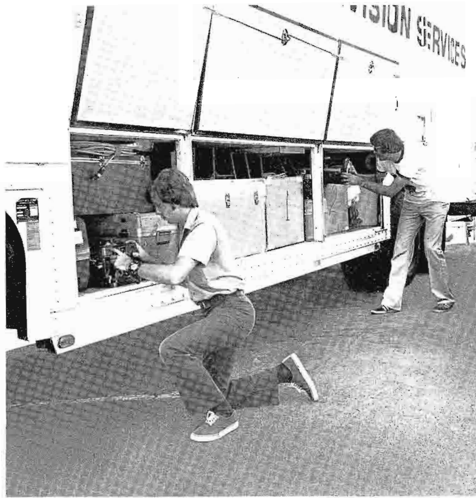
Cameras, tripods, headwheels and related equipment ride in the space between the wheels, ready for quick set-up.
